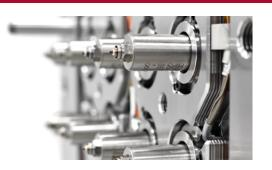
**Content:** Even when the interaction between the valve pin and the gate opening is optimised, both components are subject to wear, even in the case of non-reinforced plastics. New insights show strategies how this wear can be minimised.
