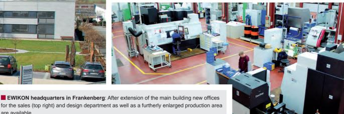
chinery over the past 10 years. It contains complex machining centres for combined turning, milling and drilling operations in one step as well as highspeed milling machines for superfinish machining and high-precision special machines to finish rotation-symmetric components.
