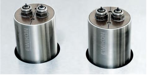
**Low-wear operation**: A special vertical groove in the nozzle body compensates for the radial thermal expansion. The valve pin load remains uncritical.
