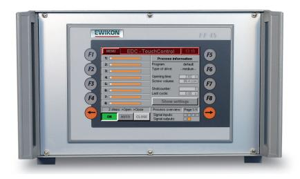
The new EWIKON electric valve gate controller system is equipped with a coloured touch screen display that allows all settings to be adjusted without requiring a laptop PC. When switching on the controller, the most important menu (F1), "process overview", is shown, giving general information about the process and the position of up to 8 drives. This menu may be entered with the "EXIT" key, available in any other menu, or after 3 minutes without touch contact.
