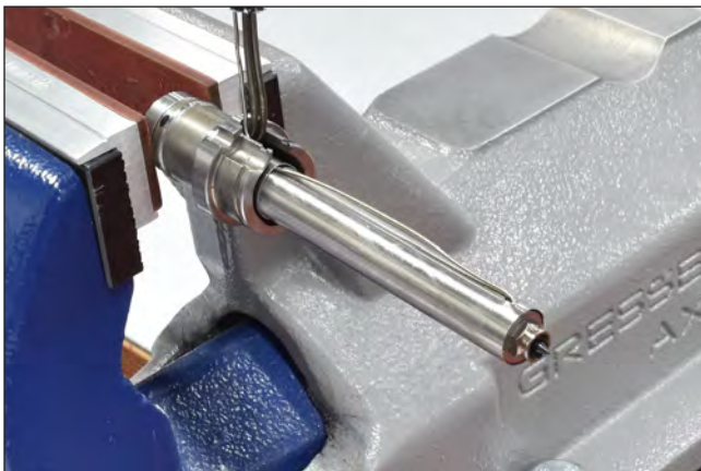
Picture 98: Pull out the protective tube
