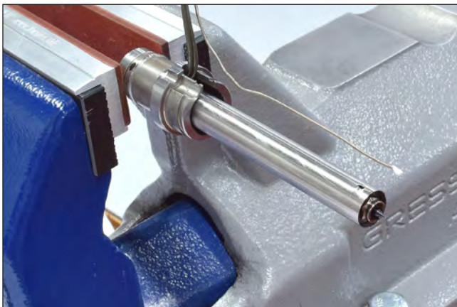
Picture 100: Coated tip of the thermocouple
