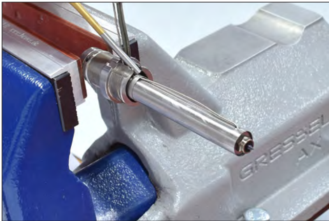
Picture 97: Pull off the clamping sleeves
