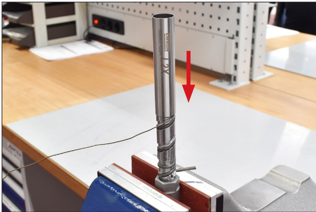
Picture 61: Installation of the new thermocouple
