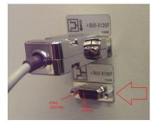
On ARBURG machines the communication pins are 4 and 5 and called "DATA#" and "DATA". Connect the communication bus to pro CONTROL as shown in the table.
