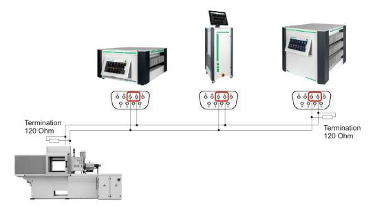
Please note, that the connection of RS485 is not standardized and each different injection molding machine may have different methods to connect the two RS485 wires. <u>Therefore</u> please carefully refer to the manual of your machine manufacturer.
