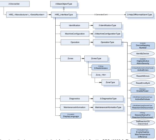
The schematic above represents the information model defined by OPC 40082-2. The pro CONTROL OPC UA server strictly follows that specification and presents the node model under DeviceSet.HRD\_EWIKON\_<SerialNumber>
